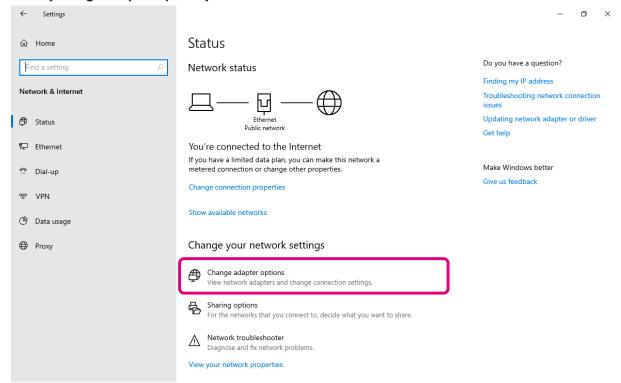
3. Double-click the network adapter (LAN card) connected to SCU-LAN10. The "**Ethernet status**" screen is displayed.
