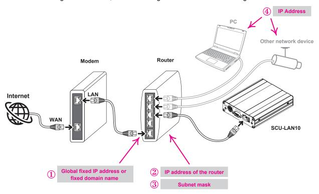
Check the following settings by referring to the instruction manual of your router or other network device. Generally, for setting routers and network devices, use a web browser such as Internet Explorer to access the IP address of the router or network device and display the setting screen.
